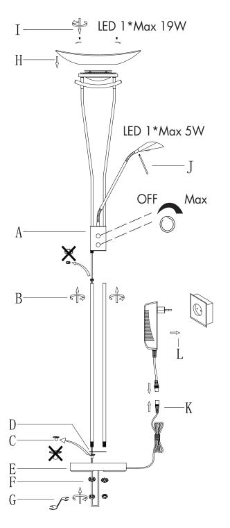
Floor lamp incl.LED QL7001066 + QL7001067 2160 +540lm Module 1512 +378lm Lamp 19W+5W LED Module 24W Lamp 220-240V~50Hz 2700K CRI>80 30000 h 15000 ON/OFF
