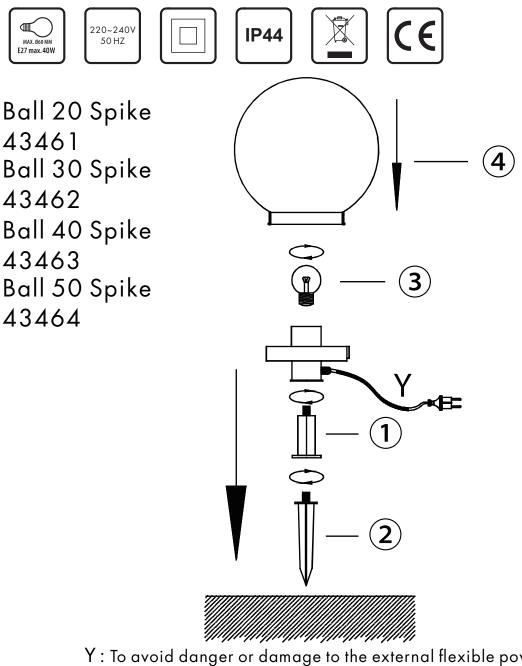
Y : To avoid danger or damage to the external flexible power cable (power supply) for this lamp may only be replaced by the manufacturer, its service representatives or a suitably qualified electrician
