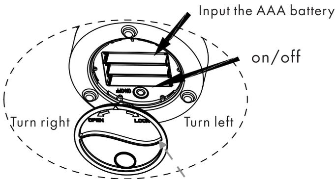
Turn the cover to the right, input the battery, and then turn left to close the cover. Press and hold the switch for 3 seconds turn off the light
