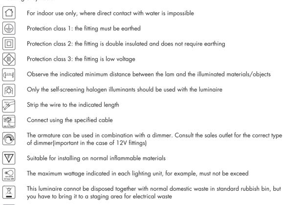
This luminaire was designed to work only with the indicated voltage
