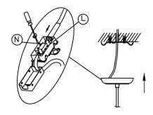
5. Fix the canopy to the wall by screws.
