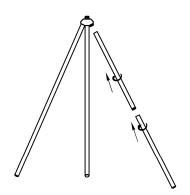
2. Connect the two straight tubes with tripod.
