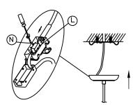
5 Fix the canopy to the wall by screws.
