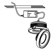
$3. Put \ the \ LED \ driver \ and \ wire inside of the ceiling .$
