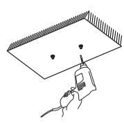
3. Fix plate to wall with screws(supplied)and make sure plate is level .
