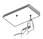
3. Fix plate to wall with screws(supplied)and make sure plate is level .
