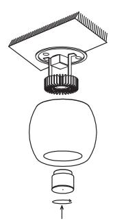
3. Fix plate to wall with screws(supplied)and make sure plate is level .
