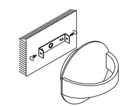
3. Fix plate to wall with screws(supplied)and make sure plate is level .
