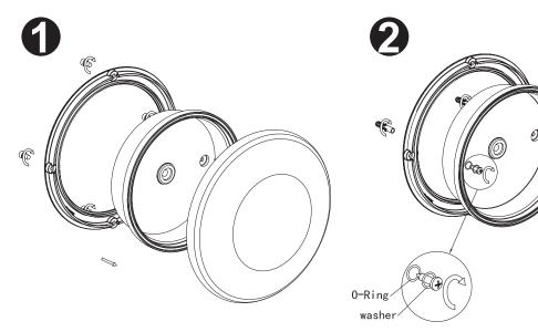
O-Ring must be under washer, No reverse position
