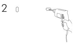
Fix plate to wall with screws(supplied) and make sure plate is level .
