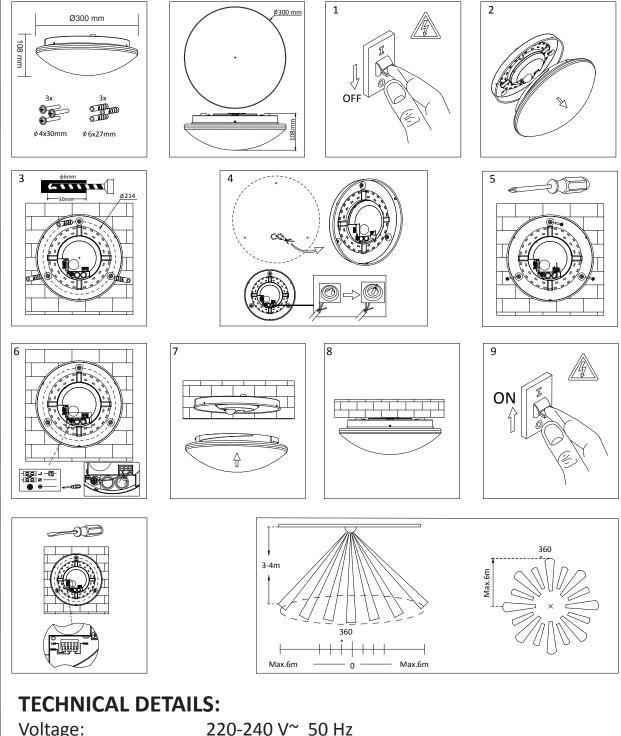
Voltage: Wattage: Detection range: Delay time: Lux control level: IP: 220-240 V~ 50 Hz 24×0.5W LED 360° and Max.6meters radius (see Figure ) 10s to 10 min. adjustable Daylight to Night adjustable 44
