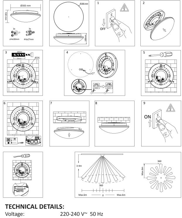
Voltage: Wattage: Detection range: Delay time: Lux control level: IP: 220-240 V~ 50 Hz 40×0.5W LED 360° and Max.6meters radius (see Figure ) 10s to 10 min. adjustable Daylight to Night adjustable 44
