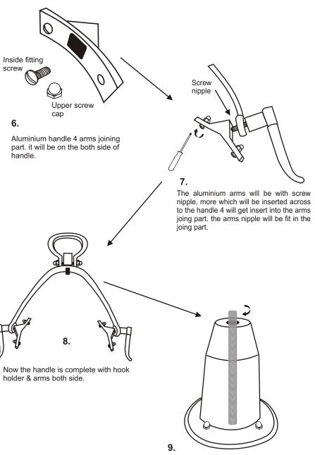
The one stud will be upper side of cap 4 one stud will be flighted from inside of the cap.
