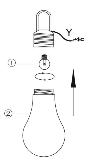
Y:To avoid danger a damaged external flexible cable (power supply cord) for this lamp may only be replaced by the manufacturer, its service representatives or a suitably qualified electrician
