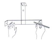
$2\,.$  Drill at the ceiling to make a hole to be match with the hook .
