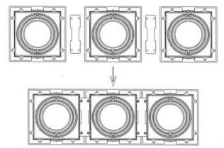
Three single units assemble with two connectors to be triple unit.
