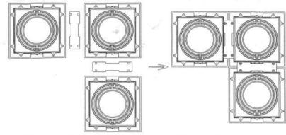
Three single units assemble with two connectors to be "L" shape triple unit.
