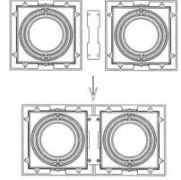
Two single units assemble with one connector to be double unit.
