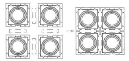
Four single units assemble with four connectors to be quadruple unit.
