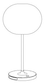
Table lamp incl. LED QL7001310 148lm Lamp 1.1W Lamp 3.7V 2500K CRI>80 30000 h 15000 ON/OFF
