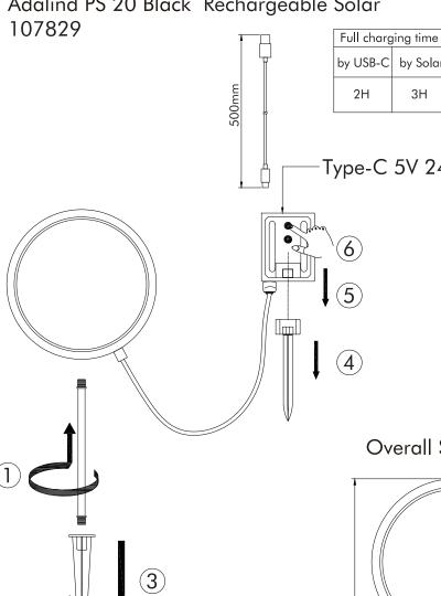
**OUTDOOR SOLAR LIGHT** 37 lm Module 26 lm Lamp 0.5W LED / 1.2W Total 3.7 Vdc Li-ion battery / 1200mAh charge voltage: 5Vdc constant voltage 240mA 2700 K / CRI >65 20000h 15000 ON/OFF
