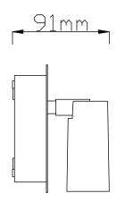
WALL LAMP incl.2xLED QL7001188 2x450lm Module 2x400lm Lamp 2x3.6W Module 2x4.5W LED Lamp 220-240V~50Hz 3000K CRI > 80 30000h 15000 ON/OFF
