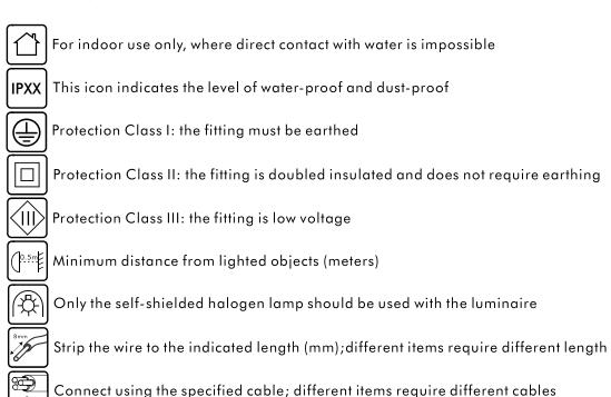
The type of lamp and maximum size and wattage indicated in each lighting unit must not be exceed; different items require different kind of light sources with different bulb icons. The armature is designed to work only with the indicated voltage. Different items require
