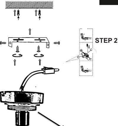
Rotate clockwise to tighten, Over tighten may cause threat to slip
